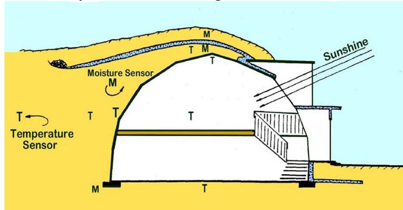
**Fig 4:** The Geodome cross-section showing the first (although small) insulation/watershed umbrella, and the locations of the important temperature and moisture sensors. [Hait J. 2005]
