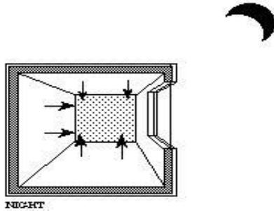
Fig 3: Transfer of stored energy at night.
