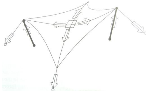
Fig2: Membrane prestressed by externally applied jacking forces
