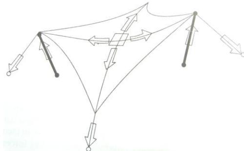
Fig2: Membrane prestressed by externally applied jacking forces
