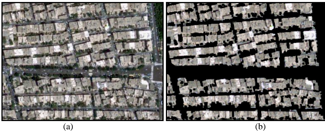
Fig 7: Building extraction, before and after: (a) Before (original image), (b) After (extracted buildings).
