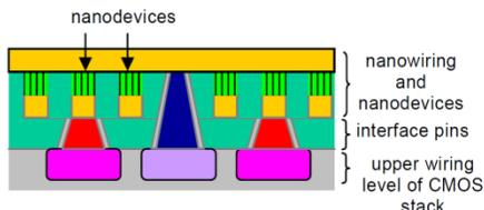
Fig. 2: Schematic side view of CMOL Interface
