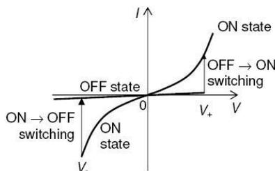
Fig. 4: I-V Curve of a nanoswitch
