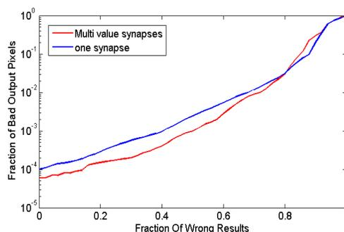
Fig. 9: Defect tolerance of a recurrent InBar
