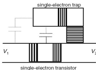
Fig. 3: Single Electron Transistor
