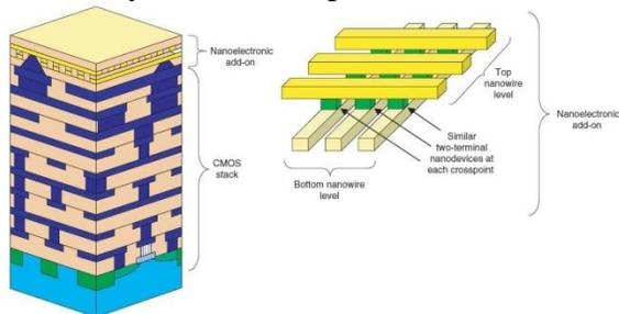
Fig. 1: Schematic of CMOL
