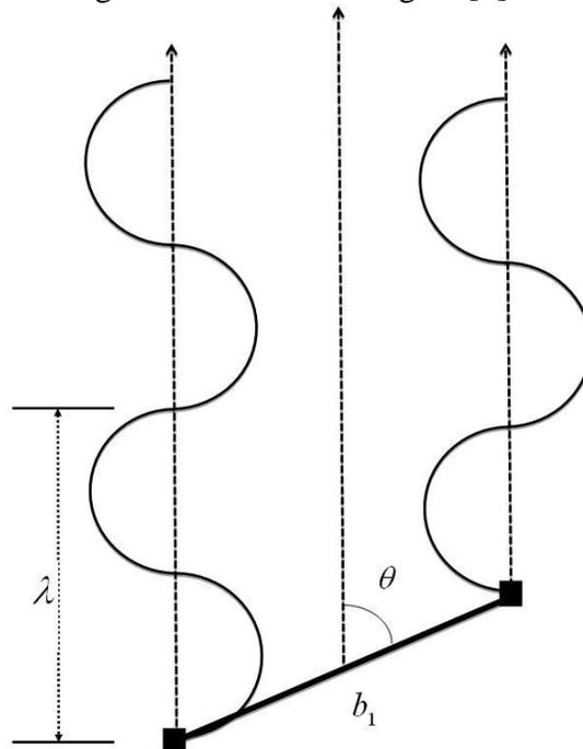
**Fig. (2)** : angle of wave front and wavelength to obtain the phase difference.
