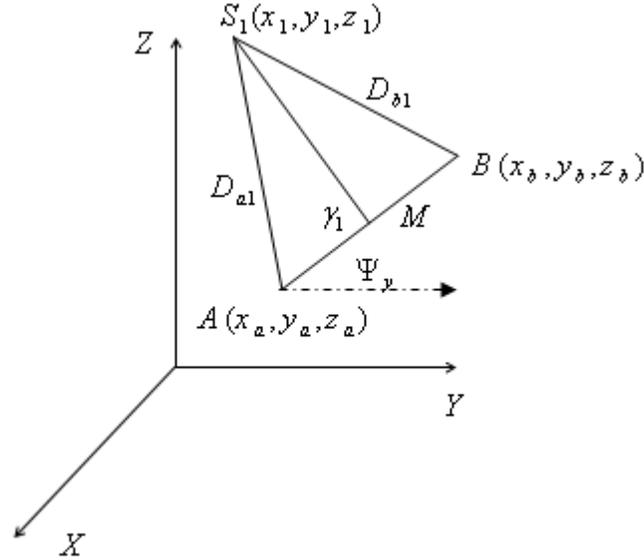
**Fig. (1):** status of antennas and GPS satellite
