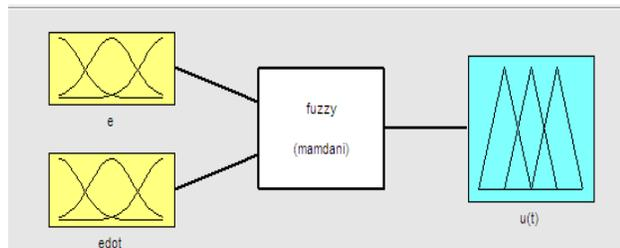
Figure 3. The fuzzy controller inputs and output
