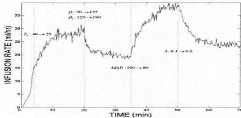
Figure 12. The system output with a IP controller
