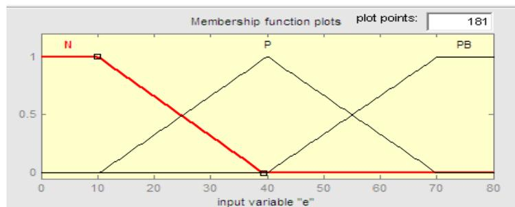
Figure 4. The fuzzy controller  $e$  input membership function
