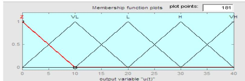
Figure 6. The fuzzy controller output membership function
