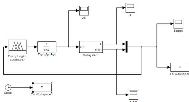
Figure 10. The system simulink using the filtrated controller
