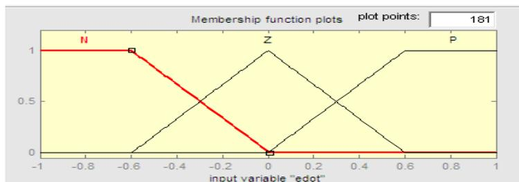
Figure 5. The fuzzy controller  $\dot{e}$  input membership function
