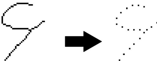
**Fig 2:** transformation of thinned image into dots
