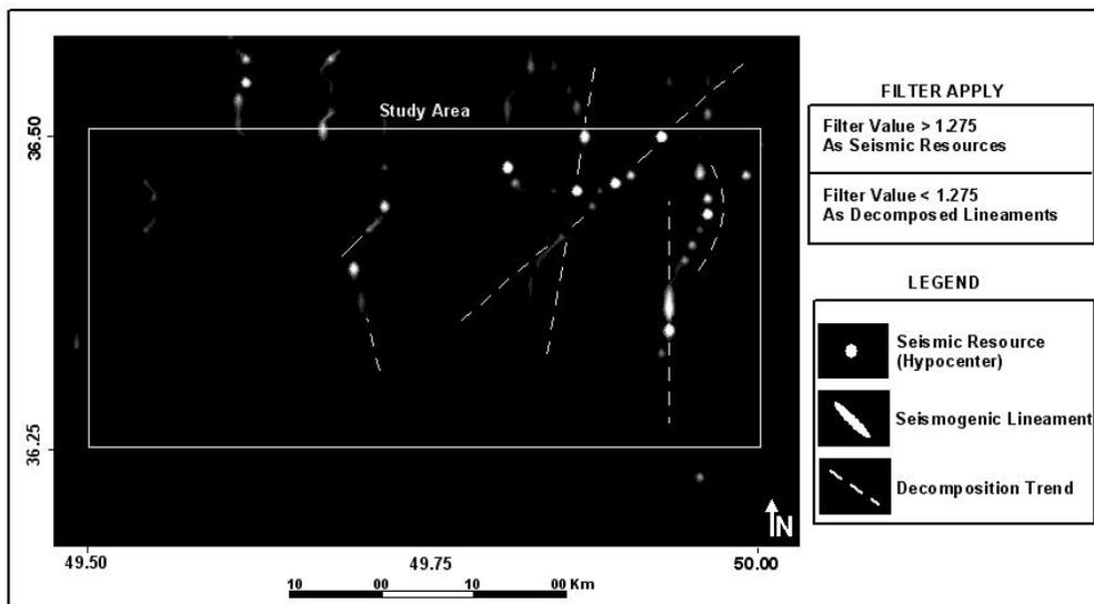
**Fig 5:** Coherent (white points) vs. Incoherent (black grounds) distribution of DN values for Seismogenic lineaments in Alamoot Sofla region (North of Iran)
