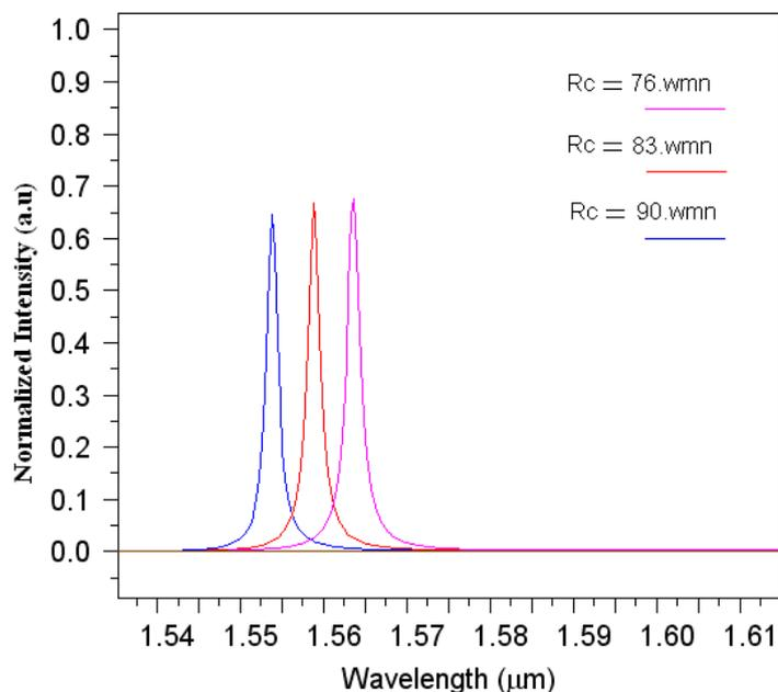
**Fig 3:** Different wavelengths selection with change the radius of defects in cavity (1564.5 nm, 1559.3 nm and 1553.5 nm for defect radiuses 76 nm, 83 nm and 90 nm respectively)
