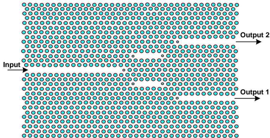
**Fig 4:** Final proposed structure for two wavelengths division demultiplexing
