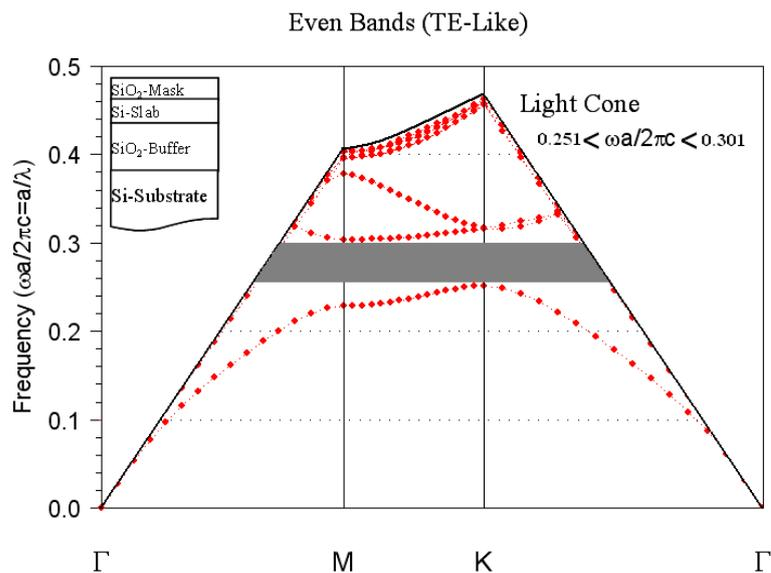
**Fig 1:** Dispersion curve for PC with  $R=115$  nm and  $a=420$  nm excited by light with TE mode.
