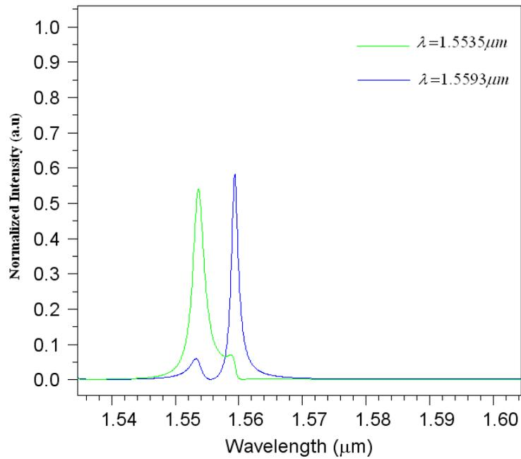
**Fig 5:** Final structure output with align radiuses of defects equal to  $R_{d1}=R_{d2}=83$  nm,  $R_{tc}=83$  nm and  $R_{bc}=90$  nm.
