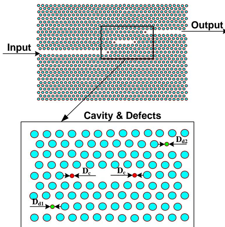
**Fig 2:** Structure with a single resonance cavity ( $D_{d1}=D_{d2}$ ).
