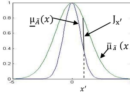
Figure 4: Primary Membership Function of Type-2 Fuzzy Set at  $x = x'$
