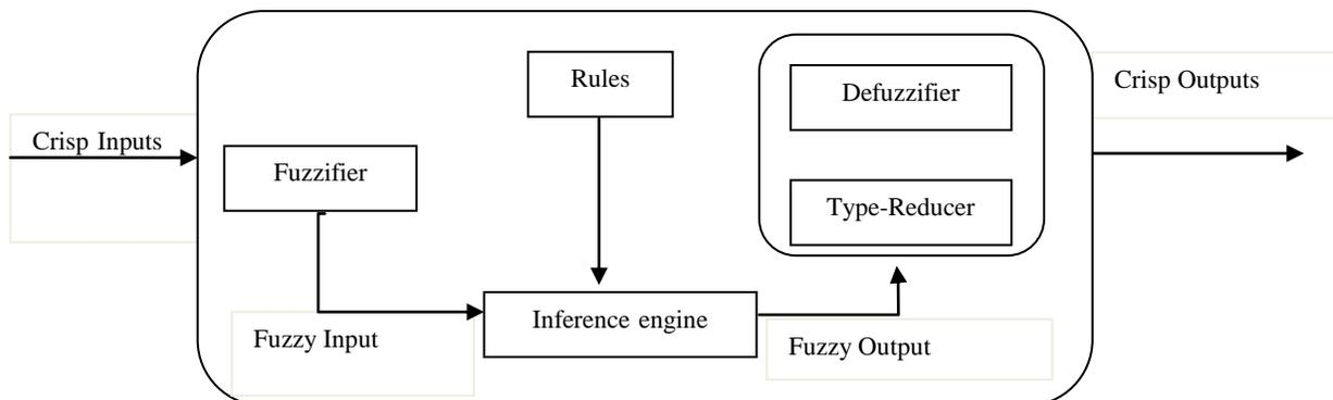
Figure 3: Type-2 Fuzzy Logic System (T2FLS) Architecture
