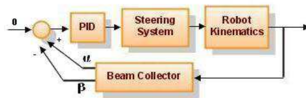
Fig. 8. The control system tries to make \alpha equal to \beta
