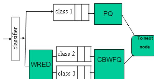
**Fig 1:** The structure of an intermediate sensor node
