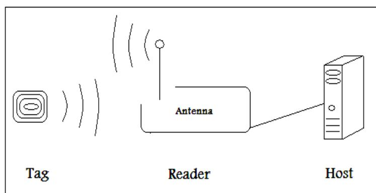
**Fig 1:** The basic components of a RFID System.
