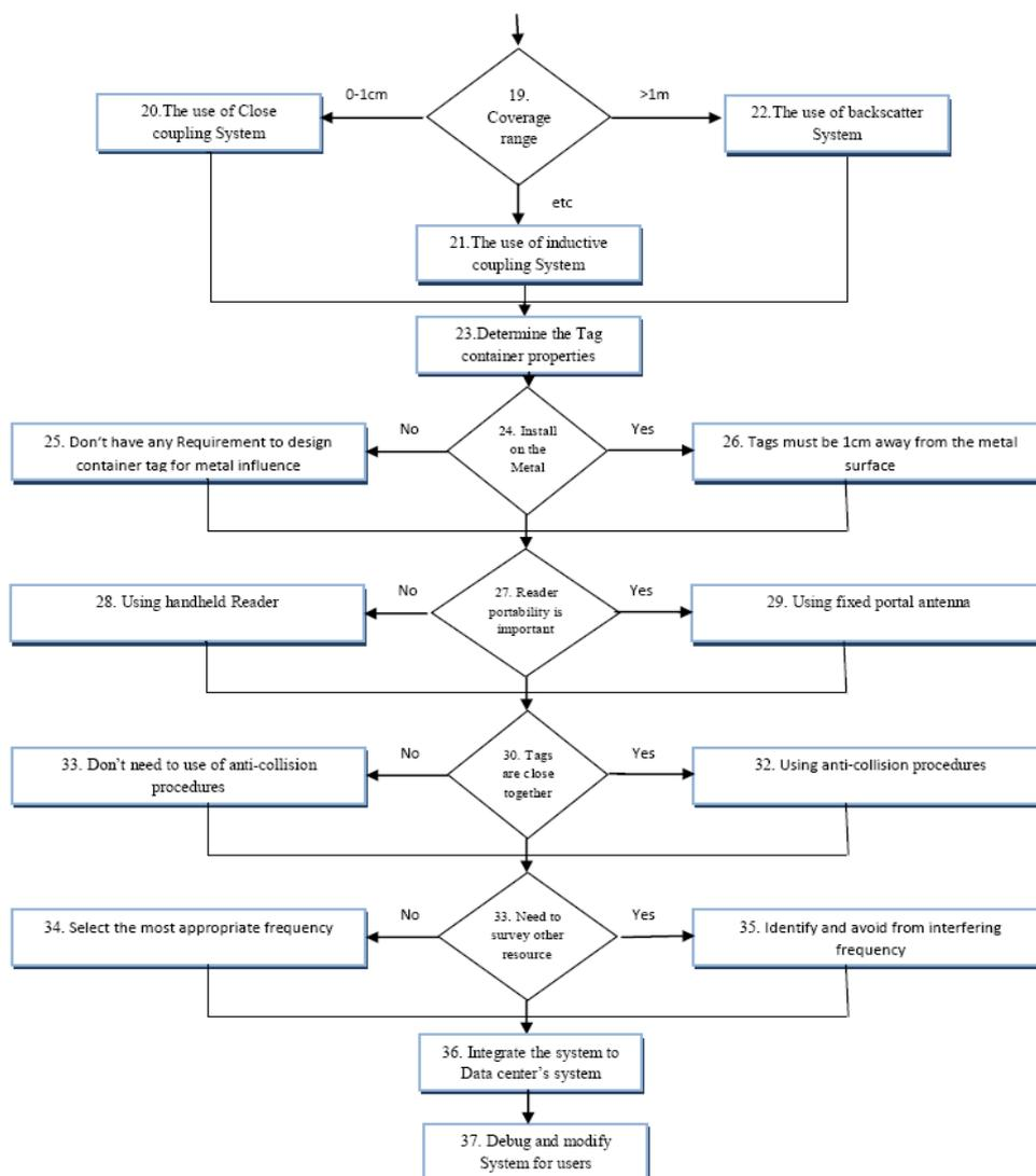
**Fig 2:** The proposed model for RFID deployment in a data center.
