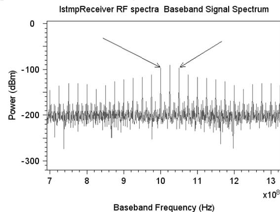
Fig.2.RF Spectra of two tone directly modulated; IMD at 1000MHz &amp; 1050MHz
