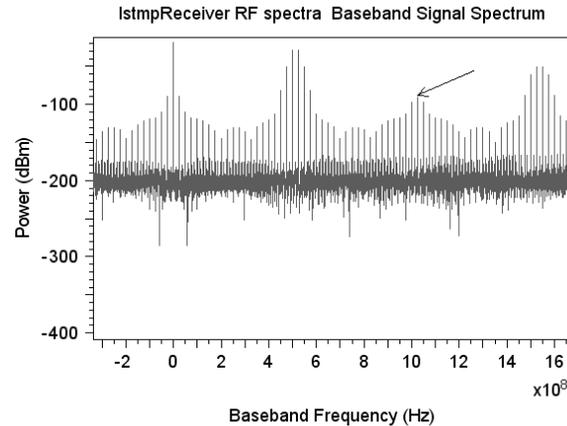
Fig.2.RF Spectra of two tone directly modulated, CSO distortion at 1025MHz
