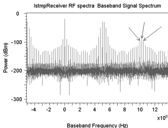
Fig.5.RF Spectra of two tone directly modulated; CSO distortion at 1025MHz, IMD at 1000MHz &1050MHz
