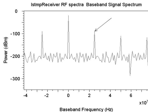
Fig.4.RF Spectra of two tone externally modulated, CSO distortion at 25MHz
