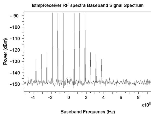
Fig.5.RF Spectra of to three frequencies directly modulated
