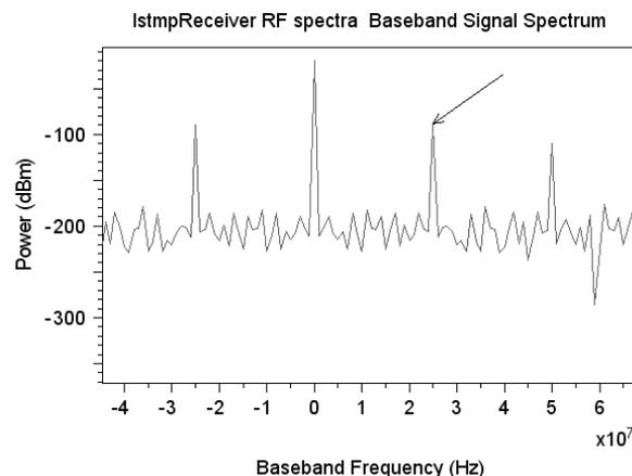
Fig.1.RF Spectra of two tone directly modulated, CSO distortion at 25MHz
