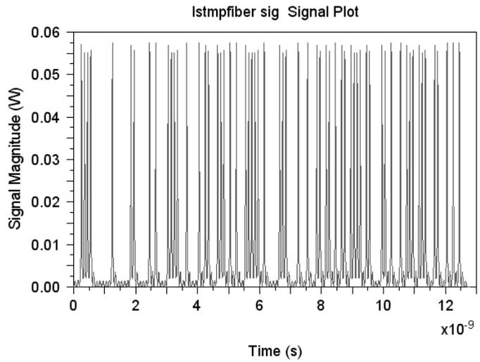
Fig.4. Signal waveform of fiber passed beam of mode-locked laser vs. time
