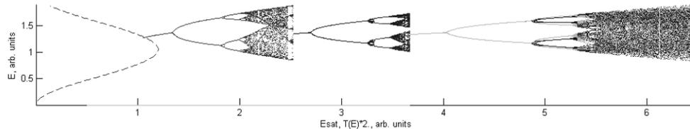
Fig.1. Bifurcation diagram of femtosecond fiber soliton laser cavity modeled on Nonlinear Schrödinger Equation
