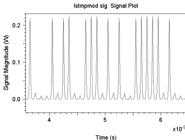
Fig.5. Signal waveform of modulated output beam of mode-locked laser vs. time in a close view
