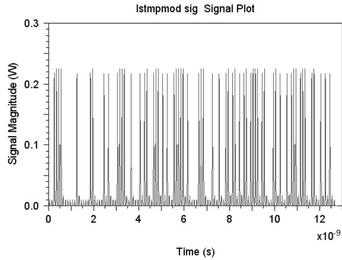
Fig.3. Signal waveform of modulated output beam of mode-locked laser vs. time
