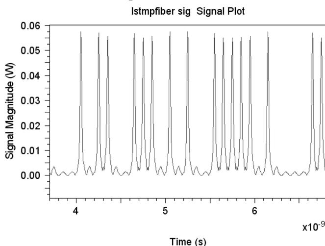
Fig.6. Signal waveform of fiber passed beam of mode-locked laser vs. time in a close view
