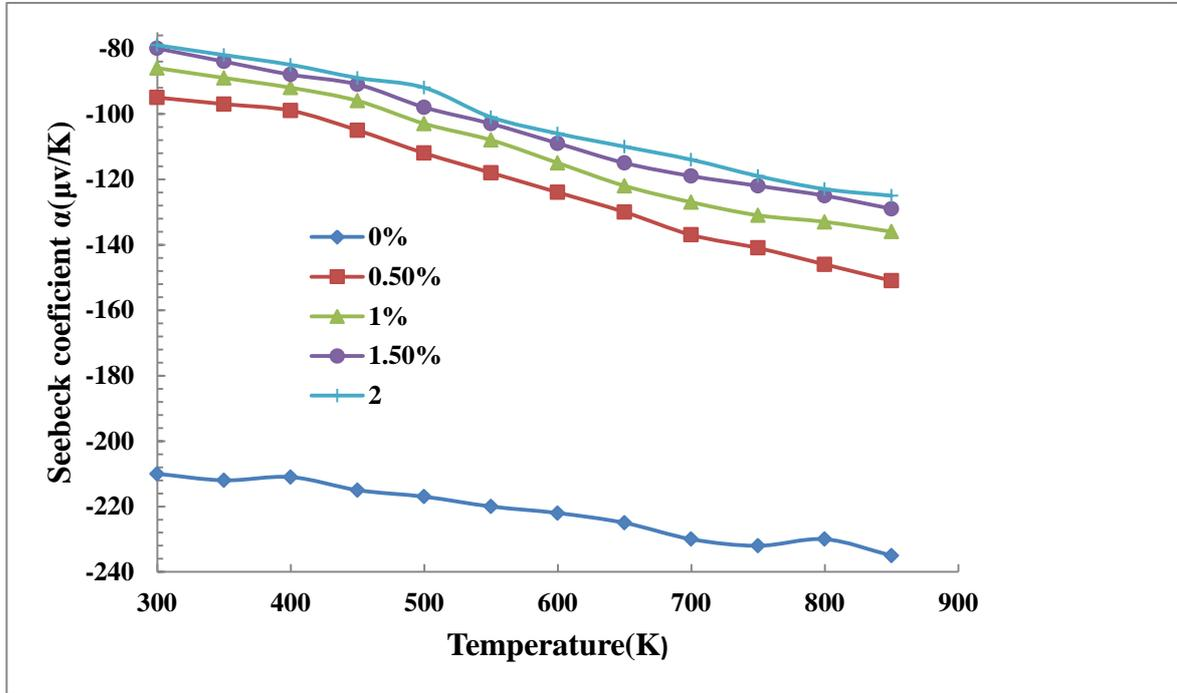
**Fig.4** seebeck coefficient as a function of temperature for the  $Zn_{1-x}Zr_xO$  samples.
