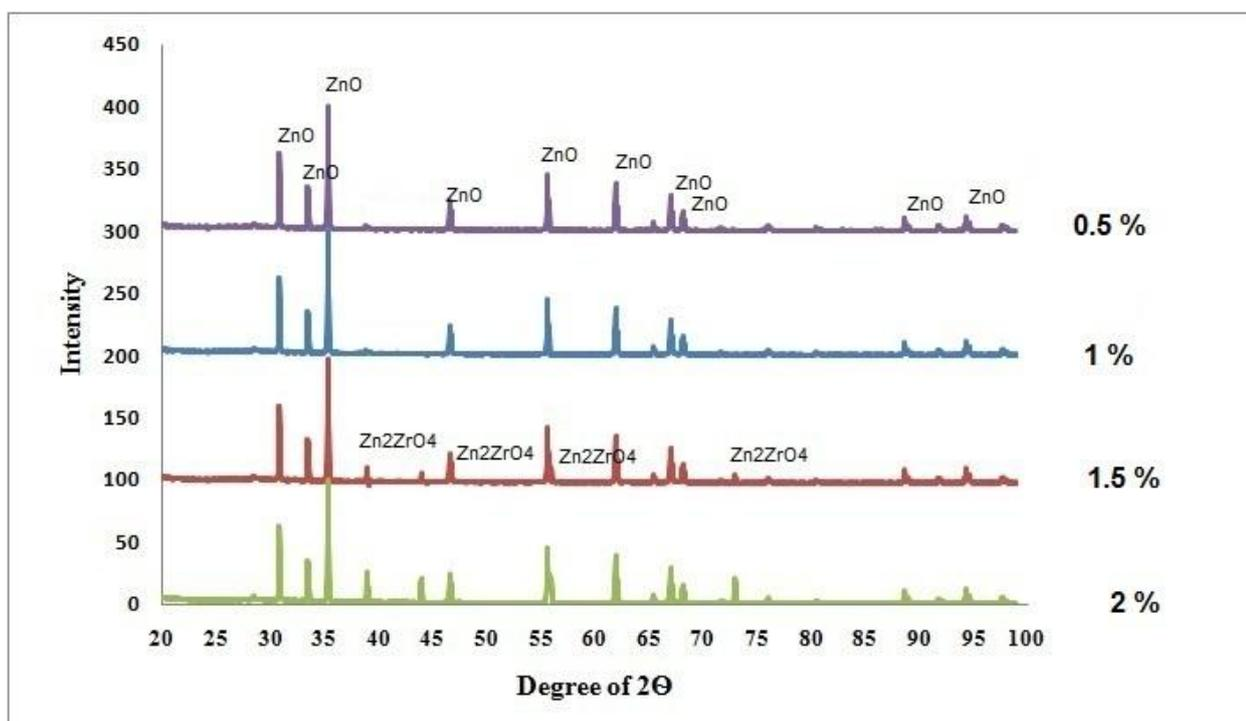
**Fig. 1** XRD pattern of the samples with different amount of ZrO<sub>2</sub> added.
