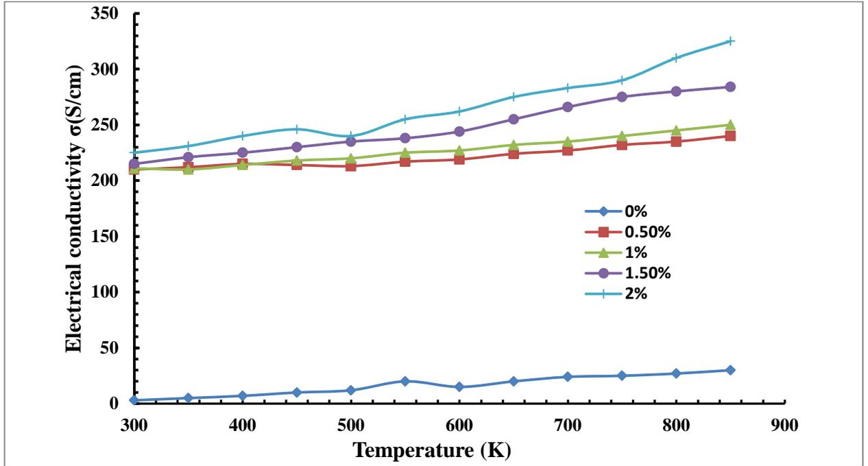
**Fig. 3** Electrical conductivity as a function of temperature for the  $Zn_{1-x}Zr_xO$  samples.
