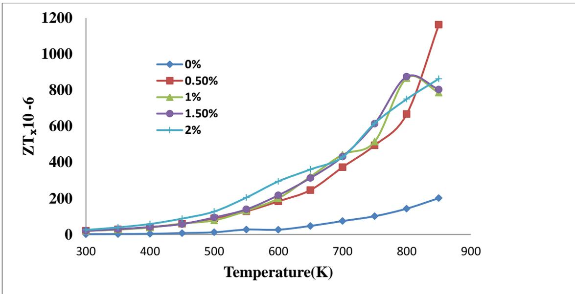
**Fig. 6** Temperature dependence of the  $ZT$  of  $Zn_{1-x}Zr_xO$  samples.
