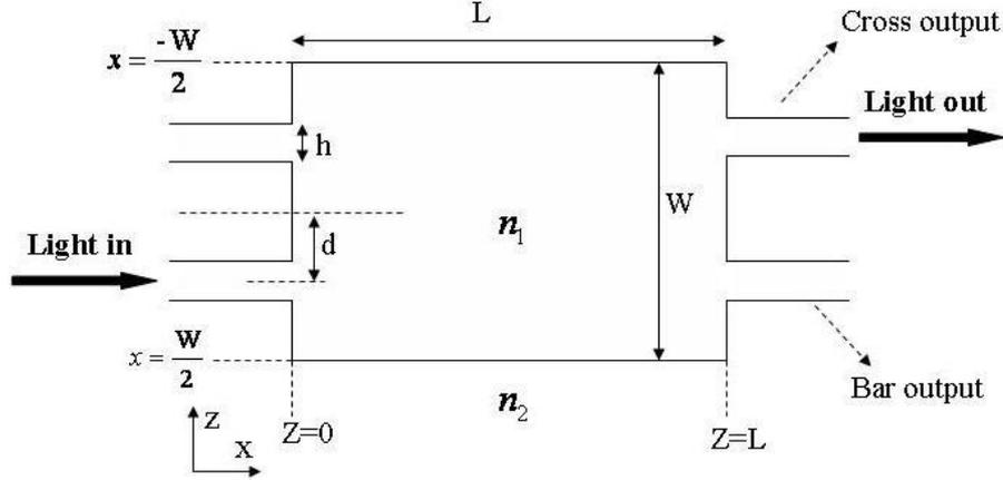
**Fig. 1:** A schematic structure of the  $2 \times 2$  MMI coupler.
