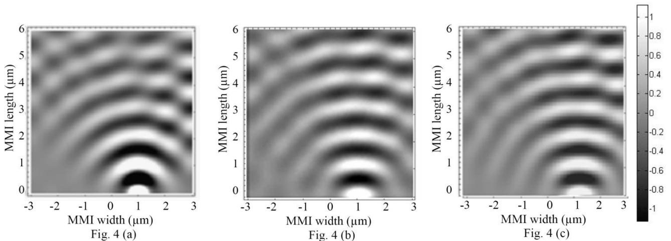
**Fig. 4:** comparison of light intensity pattern obtained by Gaussian model with those of simulation results. (a) is the result of Gaussian model, (b) simulation results by FEMLAB software,(c) simulation result by FDTD method.,(with Goos-Hänchen shift consideration). as [Mahmoodi, A. et al. (2009)].
