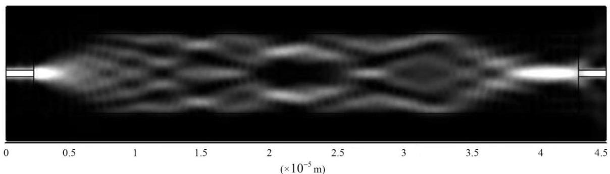
**Fig. 5:** Light intensity pattern in MMI region with the length greater than  $10\mu\text{m}$  ( $d = 2\mu\text{m}$ ) with Goos-Hänchen shift consideration.
