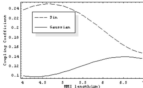
**Fig. 3:** The coupling coefficients of the MMI coupler for Gaussian and sinusoidal models with Goos-Hänchen shift consideration, ( $d = 1\mu\text{m}$ ).
