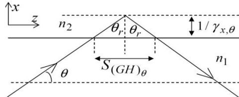
**Fig. 2:** The total internal reflection in MMI waveguide.  $S_{(GH)\theta}$  is the Goos-Hänchen phase shift and  $1/\gamma_{x,\theta}$  is the penetration depth corresponding to the  $\theta$  mode.
