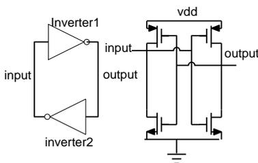
**Fig 2:** Basic Latch with transistor level.
