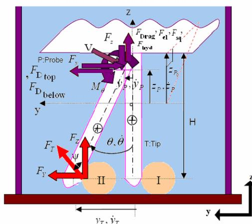
**Fig 1:** Free body diagram of AFM probe
