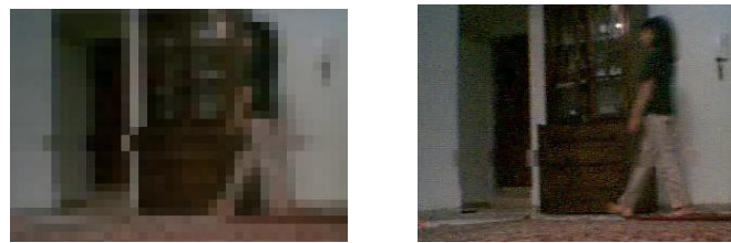
Figure 5: Frame 71 of the walking person sequence encoded at 64 kbit/s and transmitted over a GPRS channel with random error distribution and BER=10^{-4} : (a) ordinary H.264, (b) Robust I-frame coding.
