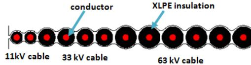
Figure 4. Slot of a 63kV powerformer with twelve cables inside it
