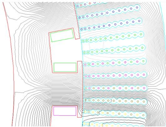
Figure 7. Flux distribution resulted from rotor excitation calculated by FEM
