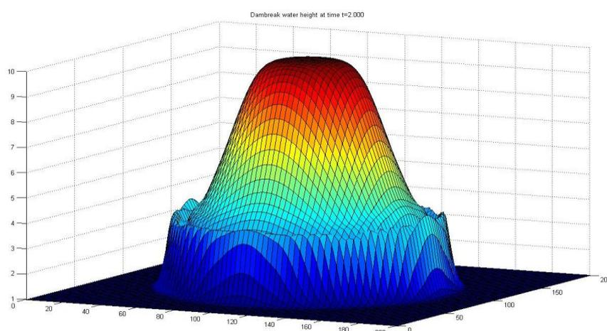
**Figure 8:**Two-dimensional solution of the circular dam break problem in a rectangular domain after 2 second based on presented model
