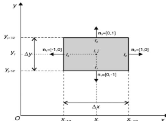
Figure2: A rectangular cell in  $x, y$  direction
