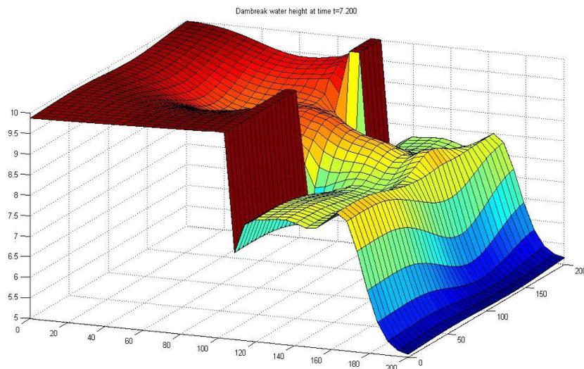
**Figure4:** Anti-symmetric dam break test in a frictionless, horizontal domain after 7.2 second based on presented model
