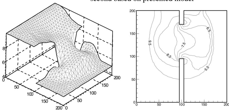
**Figure5:** Anti-symmetric dam break test in a frictionless, horizontal domain after 7.2 second
