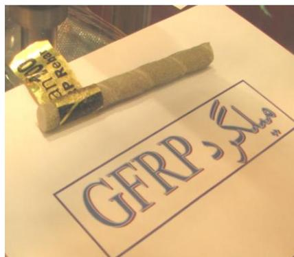
**Fig 8:** composite rebar reinforced with glass fibers
