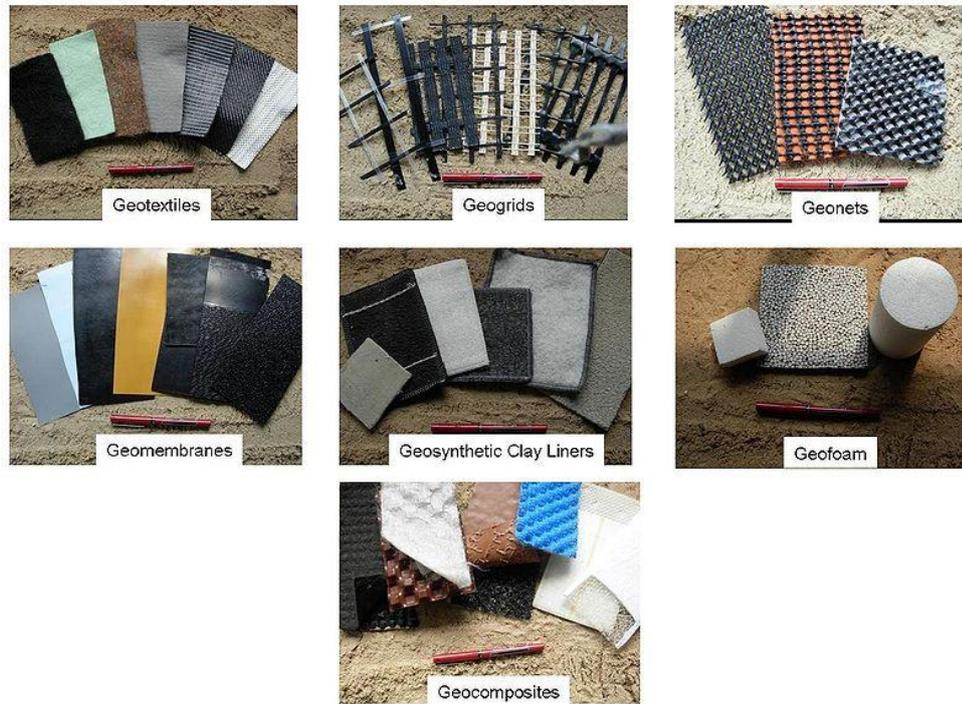
**Fig 7:** Types of Geosynthetics<sup>3</sup>
