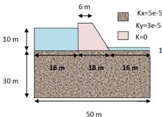
Figure2: Geometry condition of studied dam
