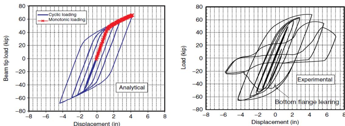
**Figure 2: Comparison between analytical and experimental results for specimen SAC3 (a) Analytical; (b) Experimental (Hedayat and Celikag (2009b))**
