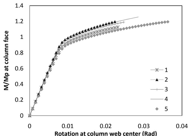
**Fig 8: Effect of parameters  $\alpha$  and  $\beta$  on moment rotation curve**
