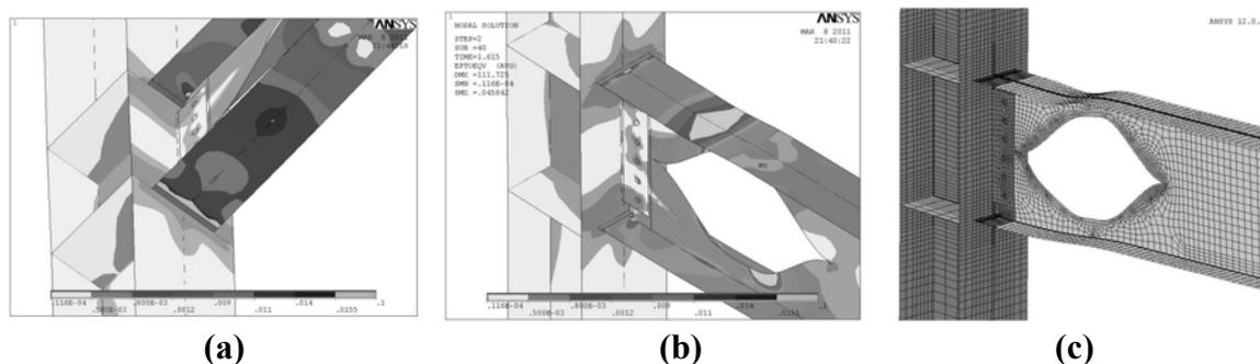
**Fig 7: Different failure modes of a modified specimen; (a) Fracture at weld access hole region; (b) Fracture at beam flange; (c) Excessive buckling of the beam flange**
