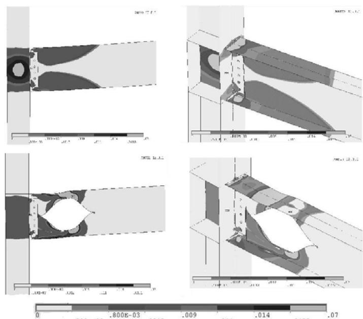
Fig. 6: Plastic equivalent strain (PEEQ) distribution of specimen SAC3: (a) Unmodified; (b) Modified
