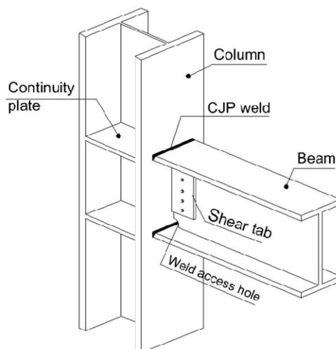
**Fig 1: typical pre-Northridge connection**
