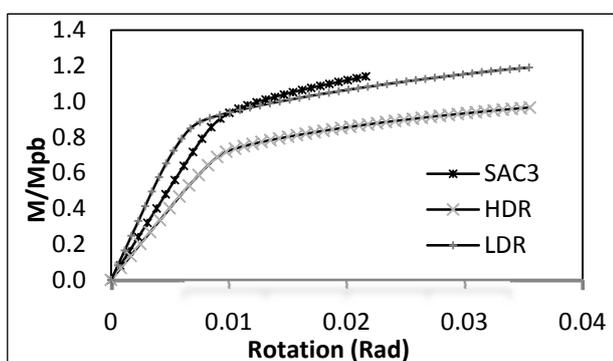
Fig 5: Normalized moment-rotation curves
