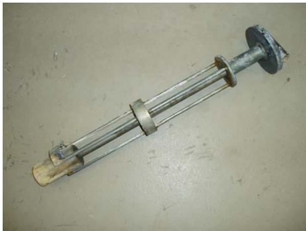
**Fig. 3** Standard compaction rammer
