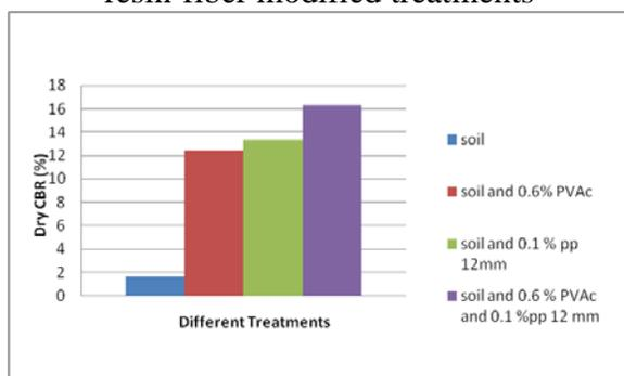
Fig 6. Comparison of optimized treatments and dry CBR results
