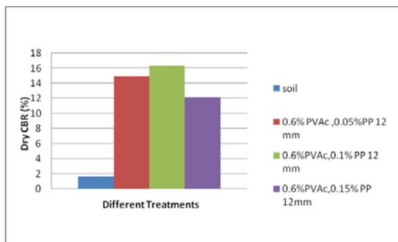
Fig 4. Effect of fiber content on dry CBR at resin-fiber modified treatments
