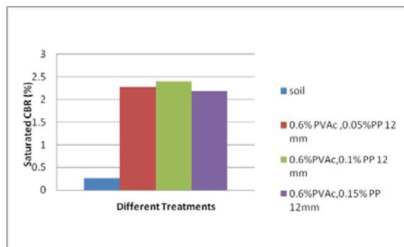
Fig 5. Effect of fiber content on soaked CBR at resin-fiber modified treatments
