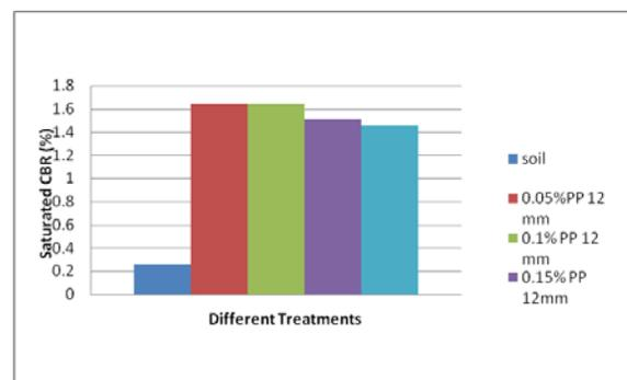
Fig 3. Effect of fiber content on soaked CBR
