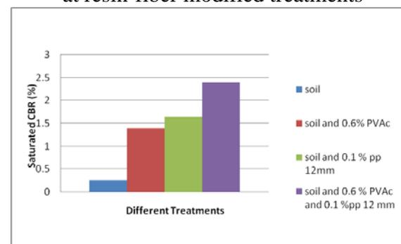
Fig 7. Comparison of optimized treatments and soaked CBR results
