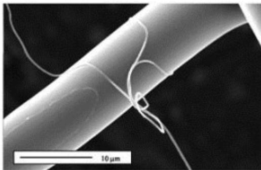
Fig 8. SEM image of electro-spun polypropylene fibers
