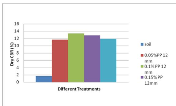
Fig 2. Effect of fiber content on dry CBR
