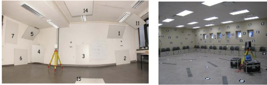
Fig1. right: Sample of a test field with point targets. left: Sample of a test field with plane targets [6]
