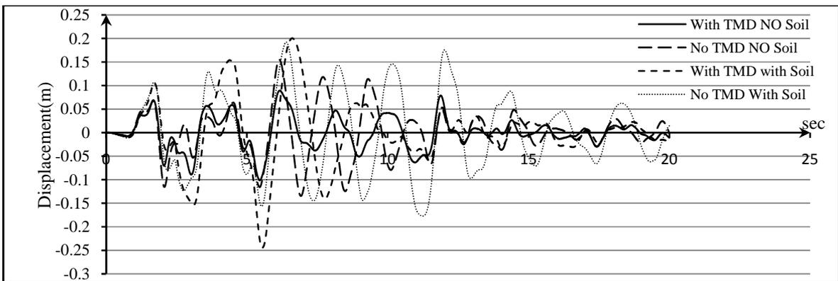
Fig 8: Top storey relative horizontal displacement (concrete frame).
