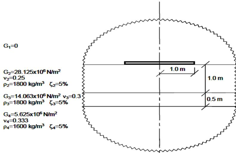
Fig 3: Surface foundation on layered site overlying homogeneous half-space [1].
