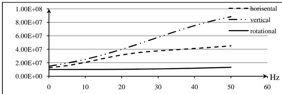
Fig 5: dynamics damping against frequency.
