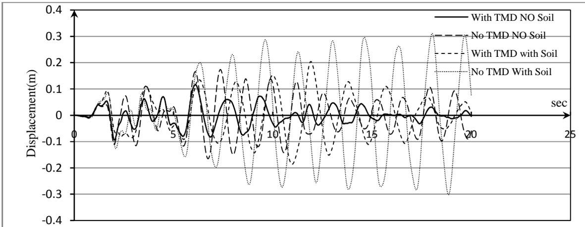
Fig 7: Top storey relative horizontal displacement (steel frame).
