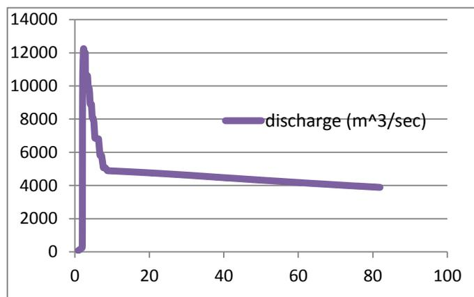
Fig. 1 The outflow hydrograph due to dam failure
