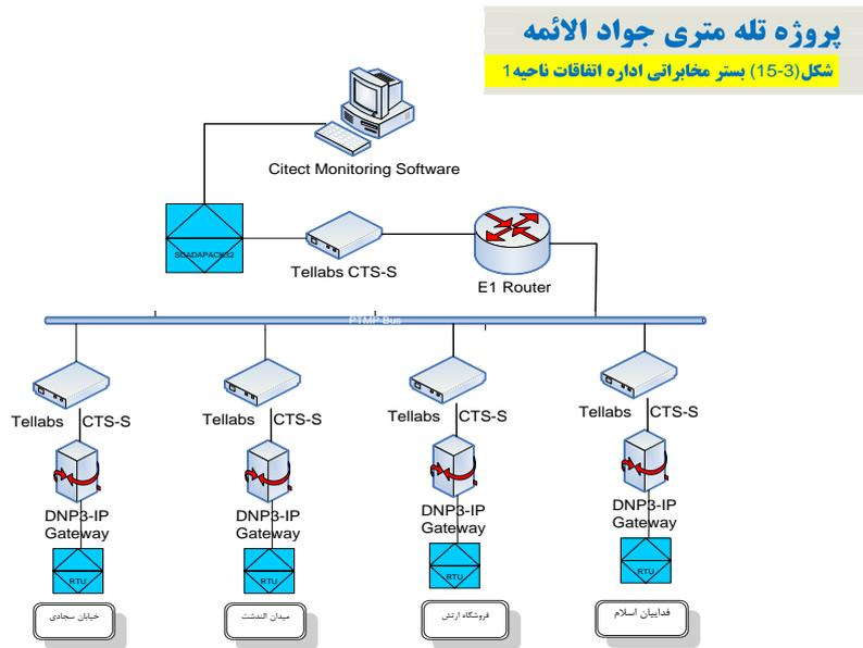
Fig. 5 Telecommunication bed between monitoring center and stations
