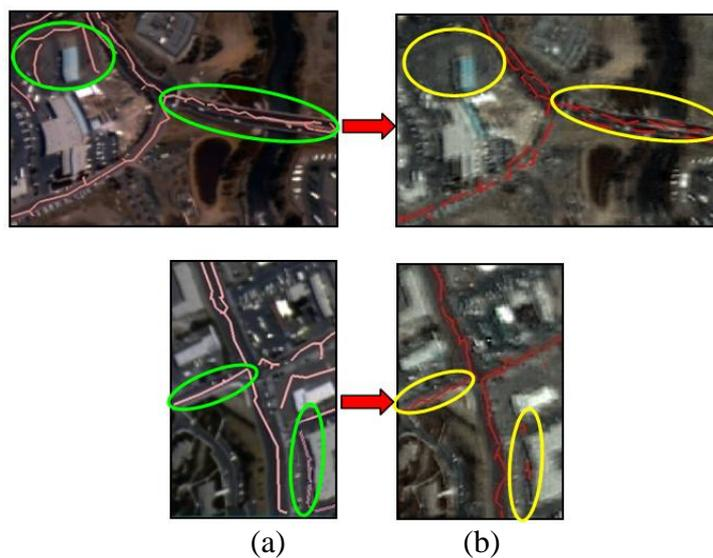
**Fig 5:** The decline of correctness and completeness value of road extraction from fused data with 1 pixel misregistration error (a: The fused data with 0 pixels misregistration error and b: The fused data with 1 pixels misregistration error).
