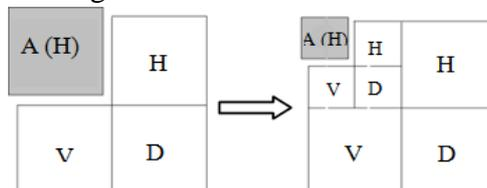
**Fig 3:** The multiscale wavelet based image fusion process
