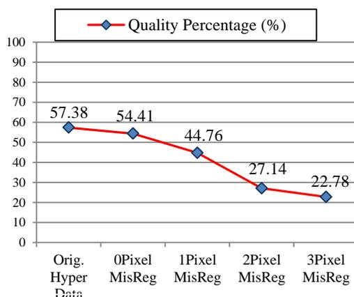
**Fig 8:** Comparison of quality percentage of extracted roads through the fused data with misregistration error and original hyperspectral images.
