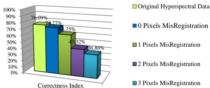
**Fig 6:** Comparison of the correctness of extracted roads through the original hyperspectral data and the fused data.
