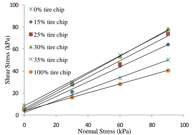
**Fig 7:** Shear stress-normal stress variation for sand-tire chip-geogrid interface with various mix ratios
