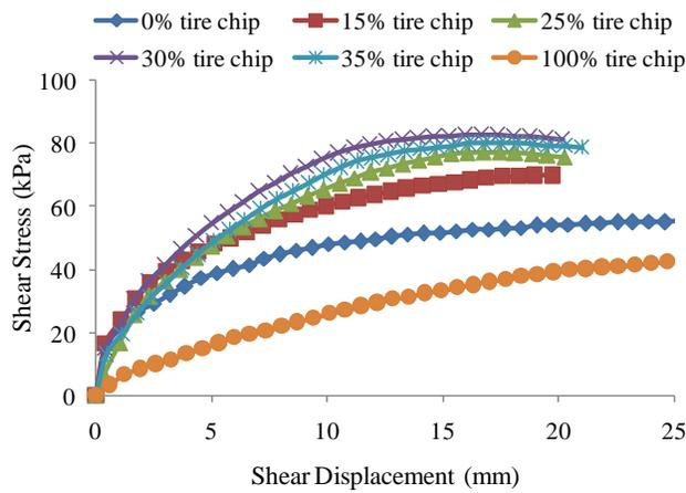
**Fig 3:** Variation of shear stress versus shear displacement for tire chip-sand mixtures at normal stress of 90 kPa
