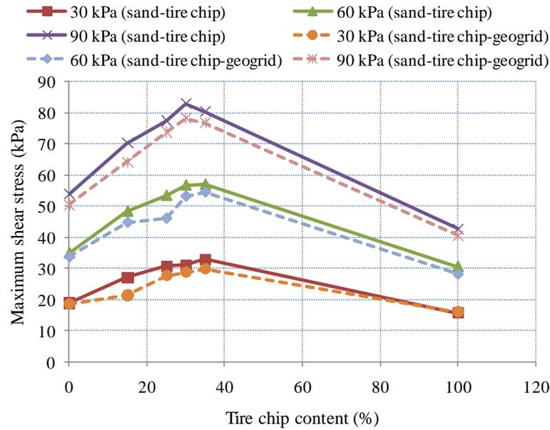
**Fig 5:** Variation of maximum shear stress with tire chip content at different normal stress
