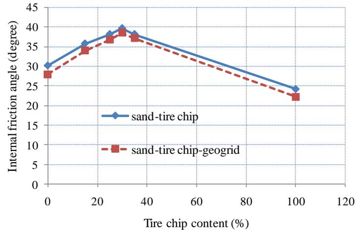
**Fig 8:** Variation of internal friction angle with tire chip content
