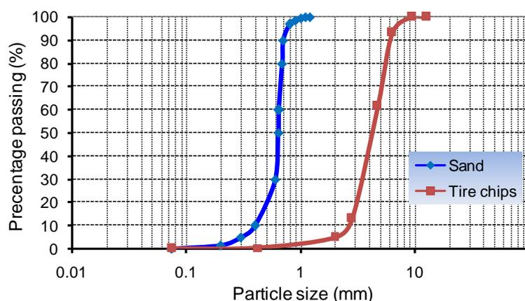
**Fig 1:** Grain size distribution of sand and tire chips
