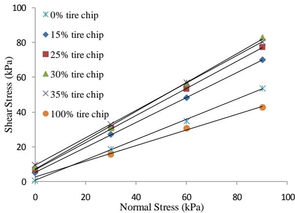
**Fig 6:** Shear stress-normal stress variation for sand-tire chip mixtures with various mix ratios
