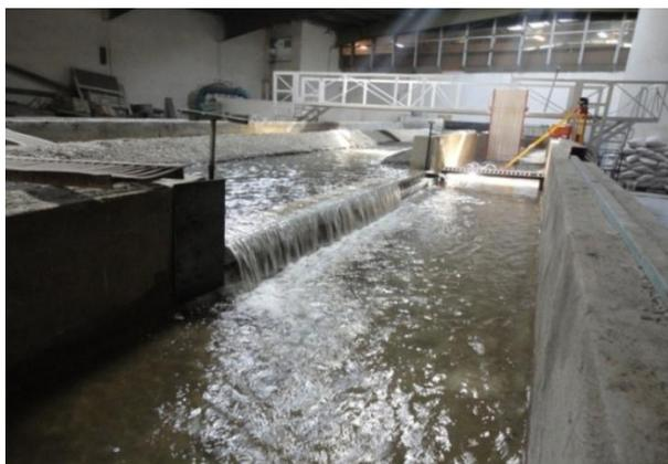
**Fig 2:** longitudinal flow profile at the side weir for discharge of 80 lit/sec
