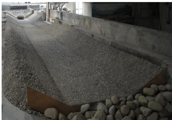
**Figure 3:** cross section of the trapezoidal main channel
