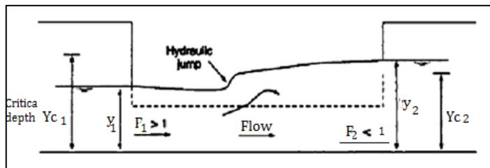
**Fig 1c:** longitudinal flow profile at a side weir under mixed flow condition
