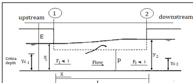
**Fig 1a:** longitudinal flow profile at a side weir under sub-critical condition
