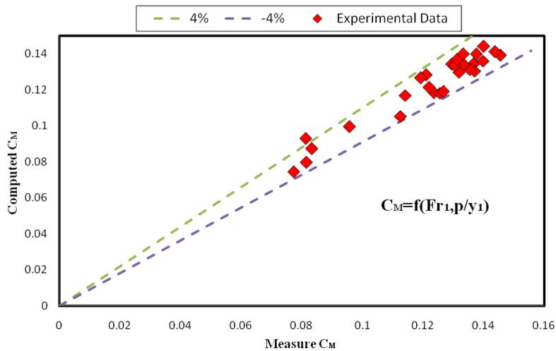
**FIG 6:** Measured Discharge coefficient versus Computed Discharge coefficient Using Eq. (16)
