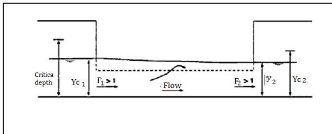
**Fig 1b:** longitudinal flow profile at a side weir under super-critical condition
