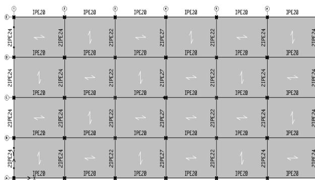
**Fig 3:** The typical floor plan of the existing structure
