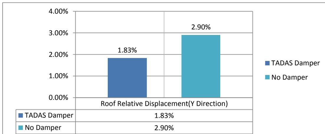
**Fig 10:** Comparison between Roof Relative Displacement in Y Direction
