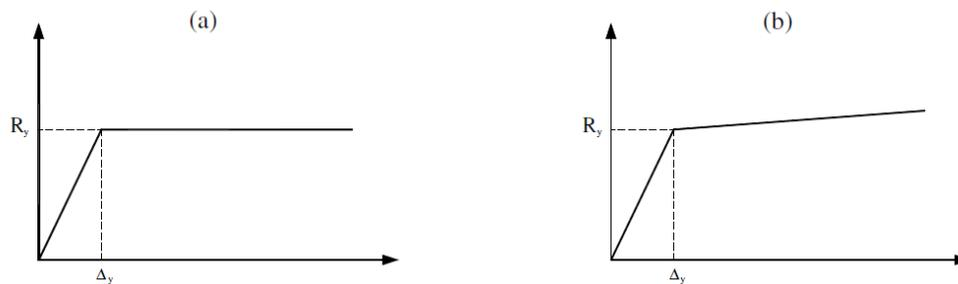
**Fig 2:** Proposed load-deformation for TADAS damper
