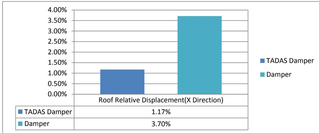
**Fig 8:** Comparison between Roof Relative Displacement in X Direction
