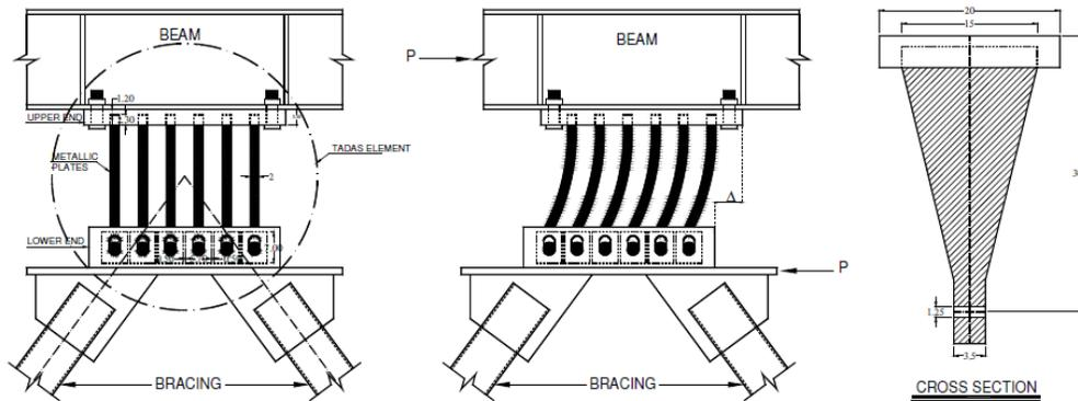
**Fig 1:** The behavior of TADAS damper during earthquake
