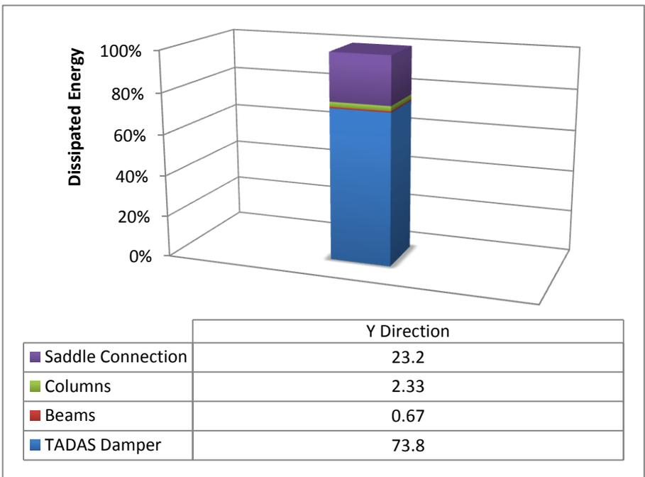
**Fig 12:** Comparison between Dissipated Energy in Y Direction
