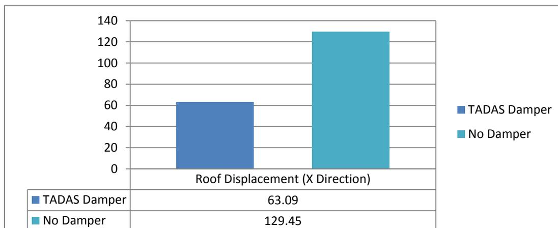
**Fig 7:** Comparison between Roof Displacement in X Direction
