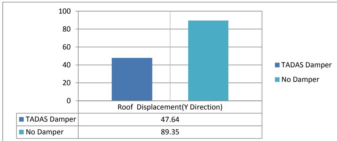
**Fig 9:** Comparison between Roof Displacement in Y Direction
