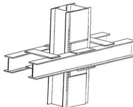
**Fig 5:** Typical saddle (bypass) connection
