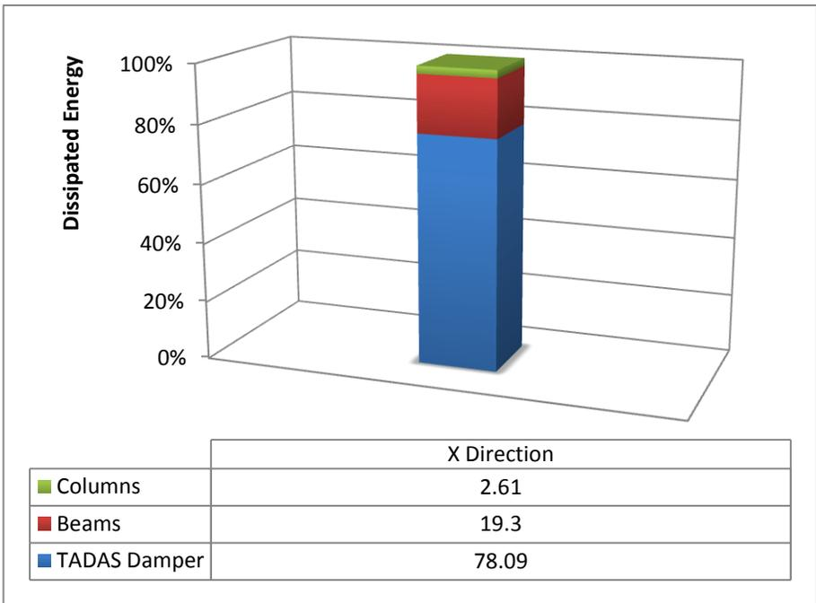
**Fig 11:** Comparison between Dissipated Energy in X Direction
