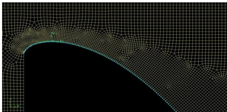
Fig 6: Meshing and the distribution throughout the model of ogee spillway.
