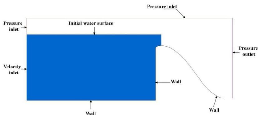
Fig 3: The Boundary Conditions of the Ogee Spillway of Simulated Numerical Model.
