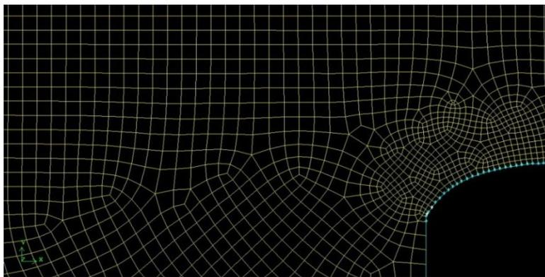
Fig 7: Meshing at the beginning of ogee spillway.
