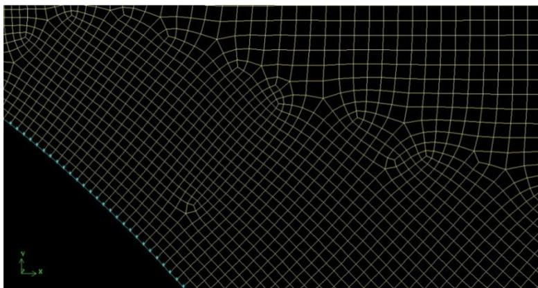
Fig 9: Meshing at the end of ogee spillway.
