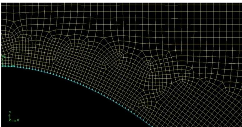
Fig 8: Meshing in the middle of ogee spillway.
