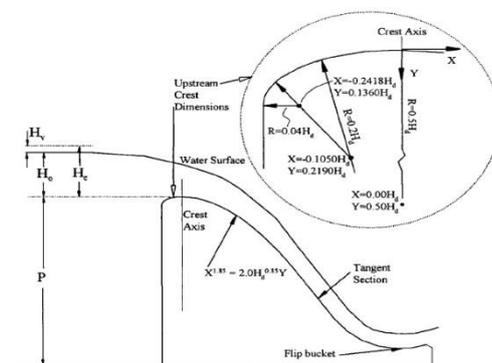
Fig 2: The Dimensions of Ogee Spillway and Flow Parameters.
