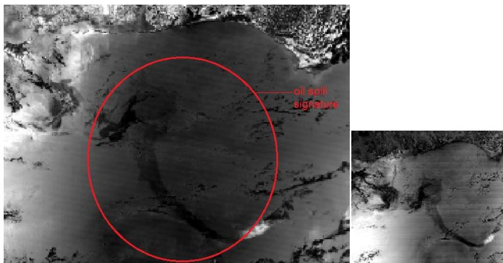
**Fig 4.** The area showing the band-ratioed image of Gulf of Mexico. The negative radiances are indications of oil spill and they are marked.
