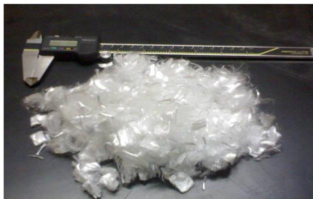
**Figure 1** Photograph of polypropylene fibers
