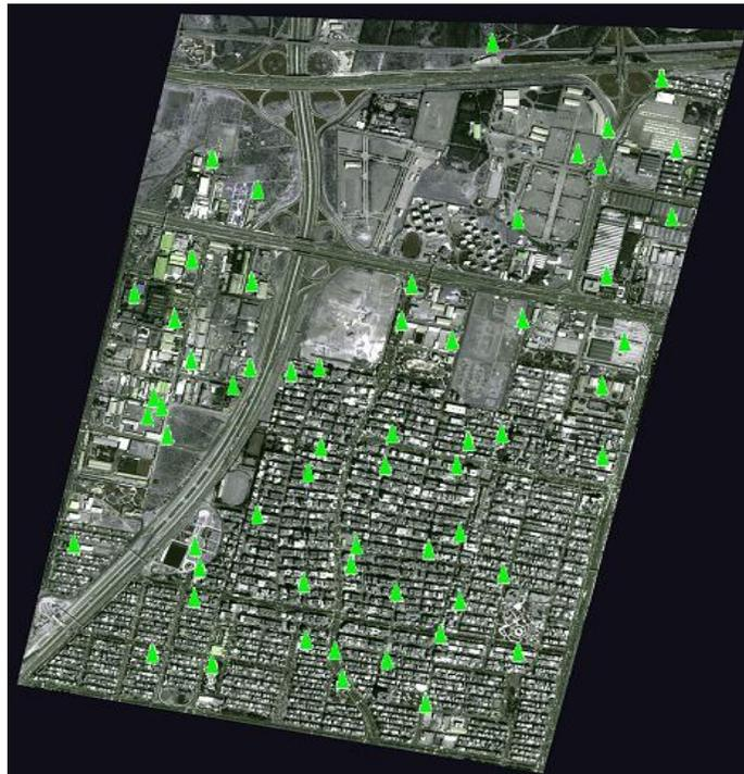
Figure 1: Geoeye\_1 image of search area and ground control points
