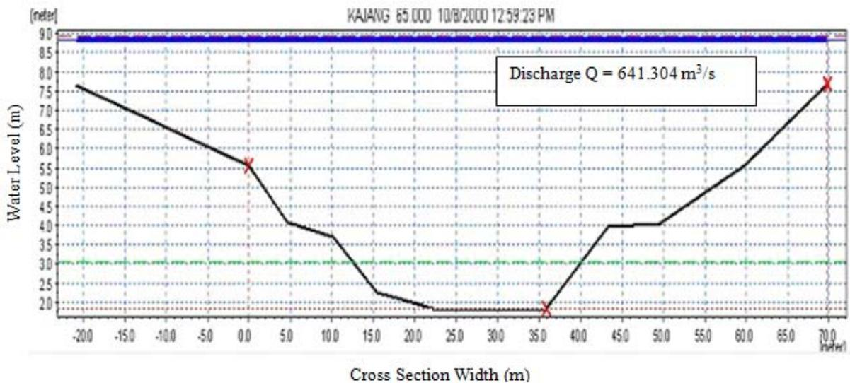
**Figure 7: Highest Water Level at Cross-section of the Simulation Point**
