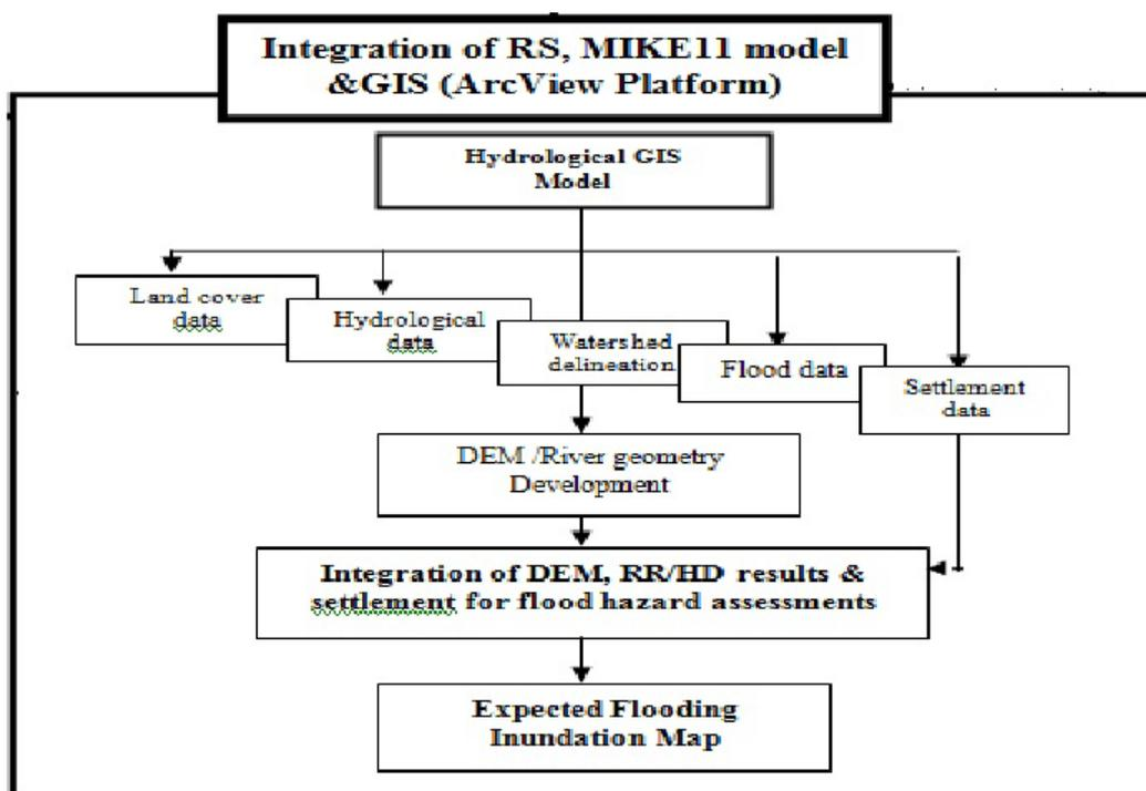
**Figure 3** Flow -chart of the Hydrological GIS
