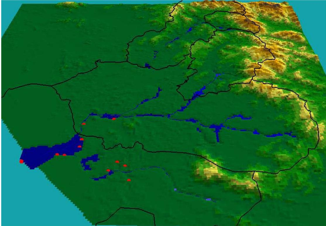
**Figure 8: Flood Map Using Runoff Results from Observed Rainfall**
