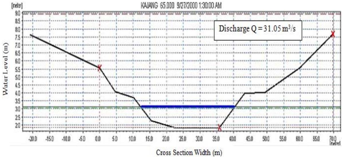
**Figure 6: Lowest Water Level at Cross-section of the Simulation Point**
