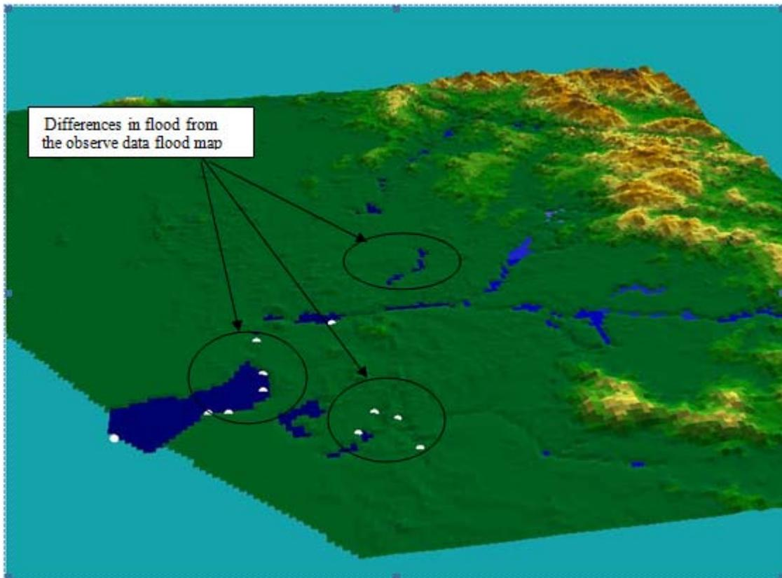
**Figure 9: Flood Map Using Runoff Results from QPF Rainfall Estimates**
