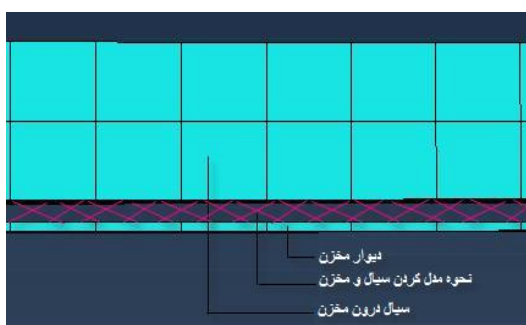
Figure 4 - magnification fluid boundaries and structure ABAQUS
