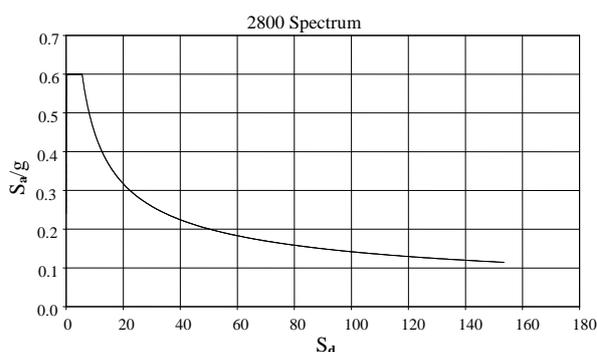
**Fig 7:**  $S_d$ – $S_a/g$  for 2800 Spectrum
