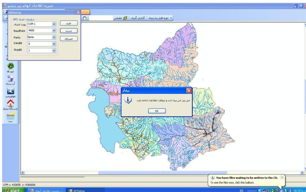
Fig. 2: View of the main window of software that shows how it communicate to a manual GPS.
