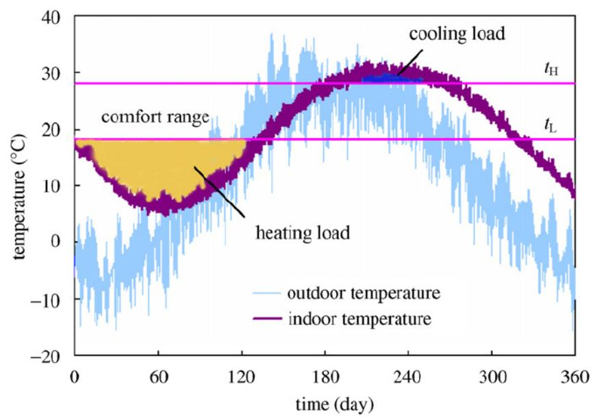
**Fig 3:** The indoor/outdoor air temperature and heating/cooling load (Zhang et al. 2006).
