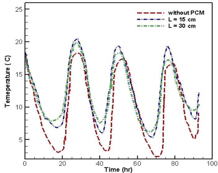
**Fig 8:** Effect of thickness of PCM and plaster wall on the temperature distribution inside the building
