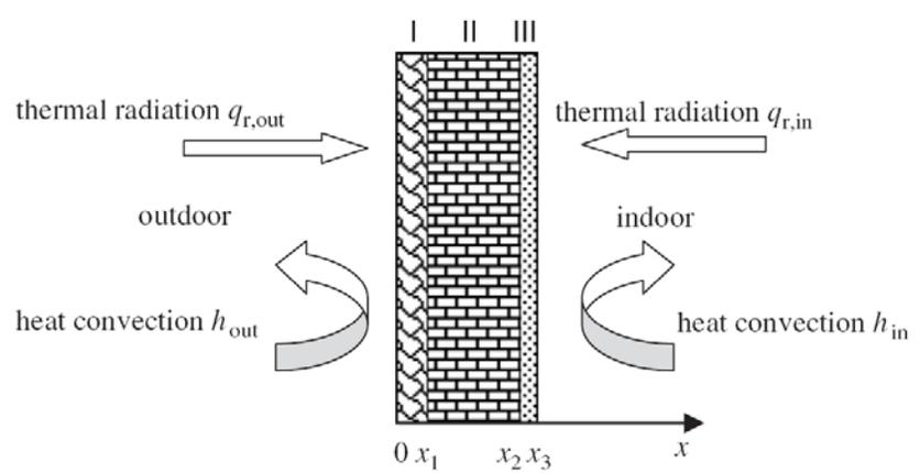
**Fig 4:** Schematic of wall's heat transfer (I, insulation layer; II, brick; III, PCM plate).
