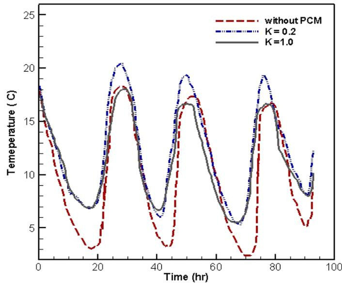
**Fig 7:** Effect of constant thermal conductivity of PCM on the temperature distribution inside the building
