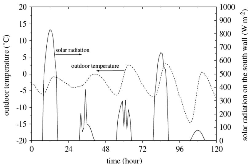
**Fig 5:** Hourly variation of outdoor temperature and solar radiation on the wall (Zhou wt al. 2008).
