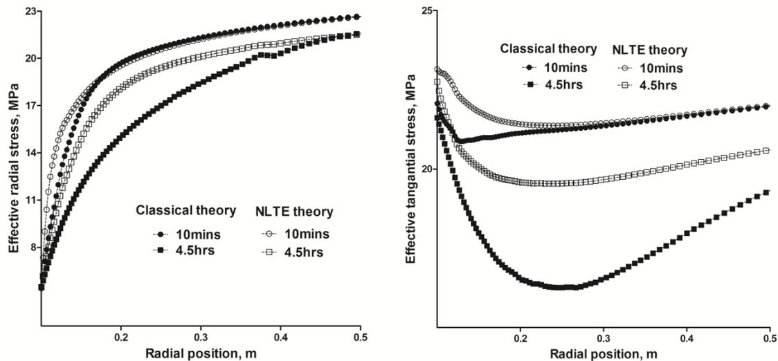
**Fig. 5.** Distribution of effective radial stress along x axis (10mins and 4.5hrs) for both cases: classical and LTNE theory.
