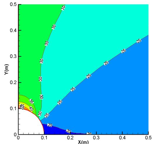
**Fig. 10.** 2D distribution of effective tangential stress after 4.5hrs for the case of LTNE theory.
