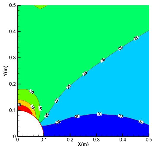
**Fig. 9.** 2D distribution of effective tangential stress after 4.5hrs for the case of classical theory.
