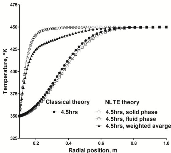
**Fig. 3.** Temperature distribution along x axis after 4.5hrs for both cases: classical and LTNE theory.
