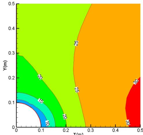
**Fig. 7.** 2D distribution of effective radial stress after 4.5hrs for the case of classical theory.
