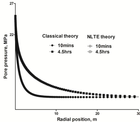
**Fig. 4.** Pore pressure distribution along x axis at two different time steps (10mins and 4.5hrs) for both cases: classical theory and LTNE theory.
