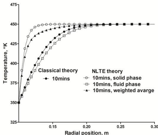
**Fig. 2.** Temperature distribution along x axis after 10mins for both cases: classical and LTNE theory.
