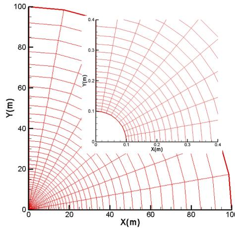
**Fig. 1.** Spatial discretization (FEM mesh of the model geometry)
