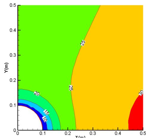
**Fig. 8.** 2D distribution of effective radial stress after 4.5hrs for the case of LTNE theory.
